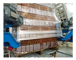
The film is cut to the appropriate length, heat sealed on the top end, and gathered on four 'fingers.' These fingers stretch the film in a horizontal (transverse) direction until the film dimensions are slightly larger than the load dimensions, then the stretched film is drawn down over the pallet, unrolling as it goes.
